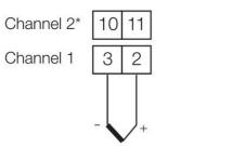
thermocouple or voltage ± 2,5 V
